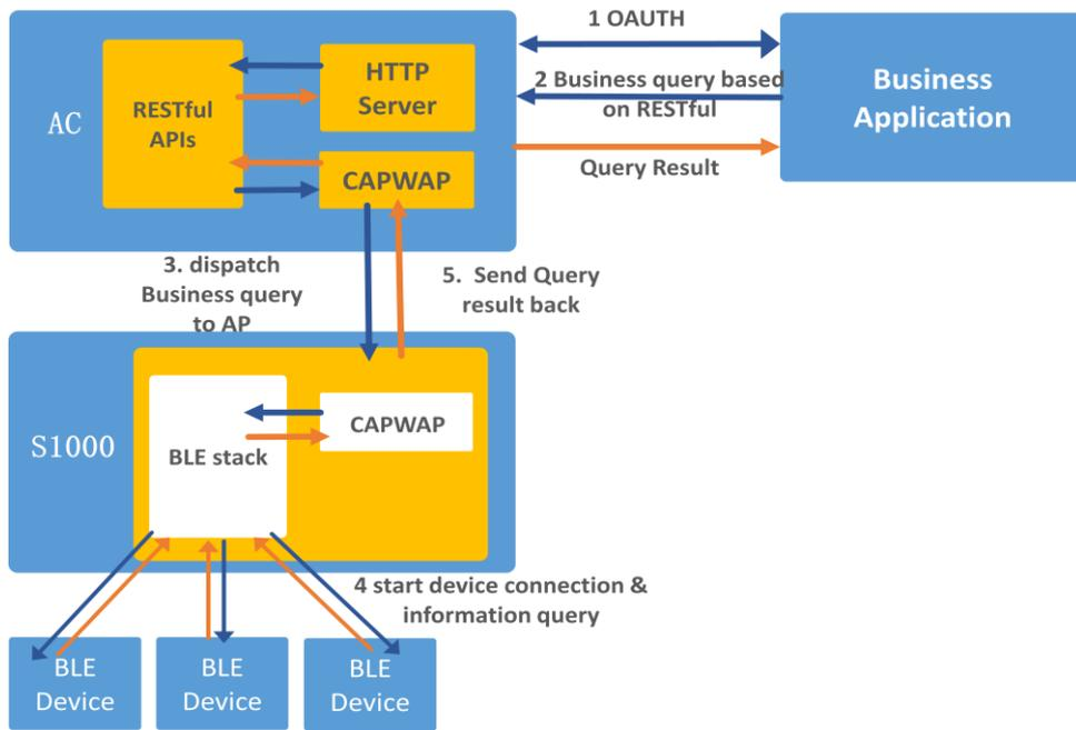
Figure 1: Cassia SDK for S1000 Working Diagram
